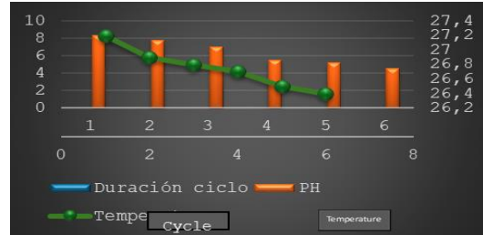
Figure 3. Temperature and pH Profile in the Reactor Using Synthetic Water During the Initial Hours of the Cycle
