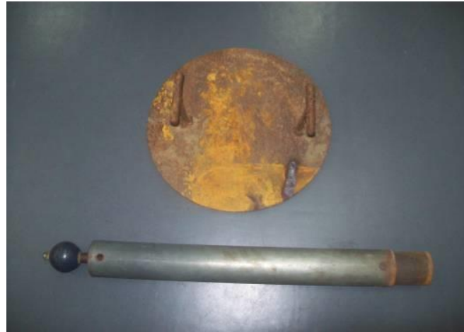
Figure 2. Proctor equipment, used to induce soil compaction.
