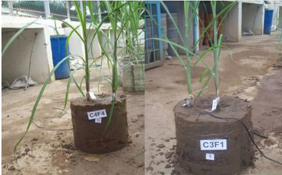
Figure 6. Sugarcane plant growth subjected to 36 blow compaction level and every three-day-irrigation (C4F4) and 24 blow compaction level and interday irrigation (C4Fi).
