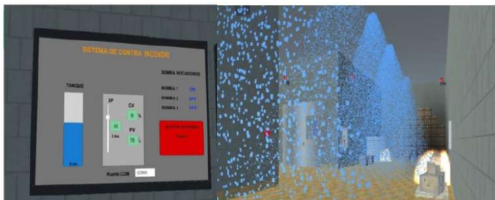
Figure 16. Simulation of Fire in Zone 1 and ignition of water sprinklers.
